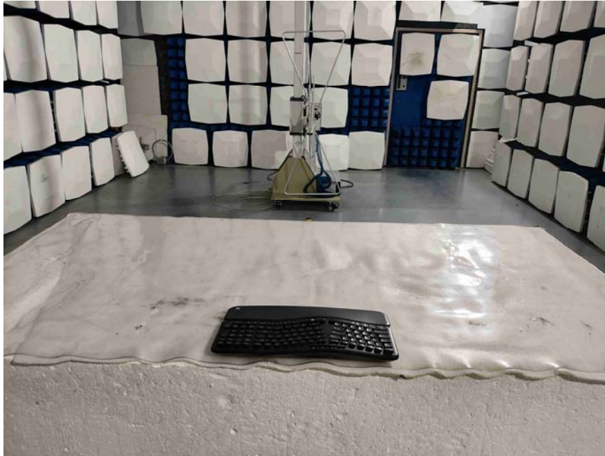
Radiated emission test view
